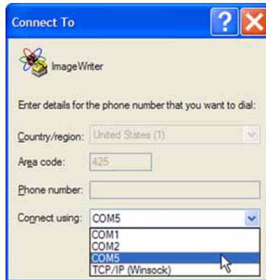
Figure 2-16— ImageWriter Will Usually Be the Highest Number COM Port If You Just Plugged It into Your Computer
