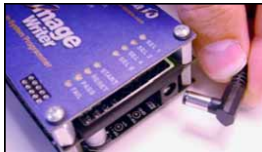
Figure 2-2—Plug AC Adapter into Auxiliary Power Connector
