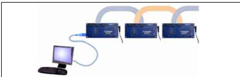
Figure 2-13—Link Networked ImageWriter-300s : One Master IW-300 and up to 31 Linked IW-300s
