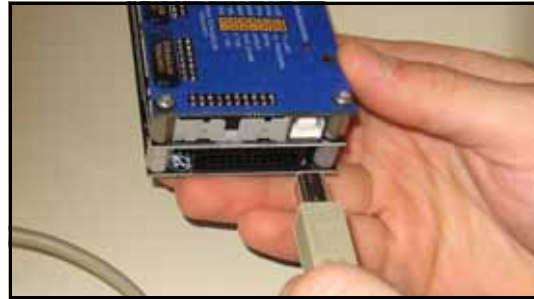
Figure 2-14—Plug the USB Cable into Master IW-300
