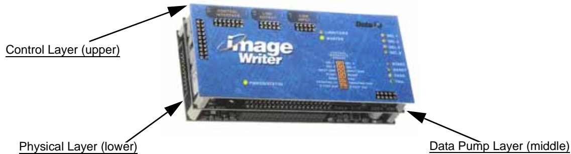
Figure 1-5—IW-300 Showing Three Layers of Hardware
